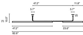
(1) The height can be increased by means of the 40 or 60 cm poles (max. 3 units per each side). They can be combined.
