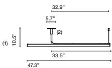
(1) The height can be increased by means of the 40 or 60 cm poles (max. 3 units) They can be combined.
