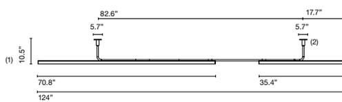
Aluminum structure. Methacrylate light tube.
