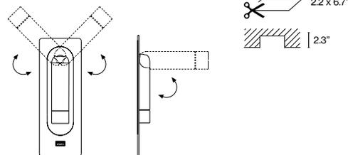
The orientable wall lamp is easy to use as the light turns on automatically when the Ledtube is opened, and turns off when it is closed. Honeycomb grill to avoid glare.
